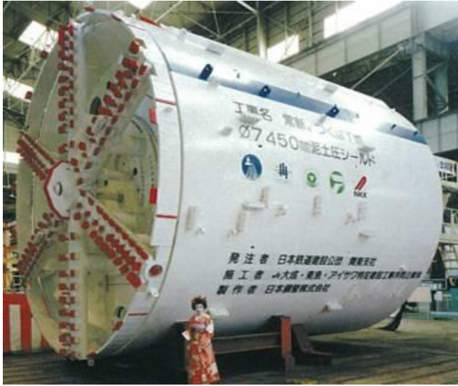
EPB TYPE TBM
